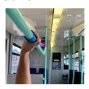
In just a few weeks, the experts at K-Profile developed the clip-on tube together with the customer. In this process, K-Profile uses the 3D printers available in the company for the first prototypes. The design of the profiles and extrusion tool is done using CAD, so that the tools are manufactured in the shortest possible time in the company's own tool shop.
